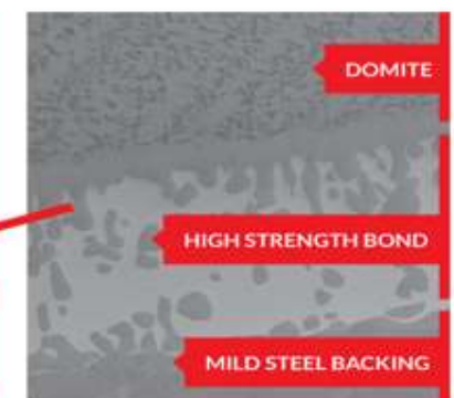
300X ZOOM BOND SHEAR STRENGTH 225 MPA
